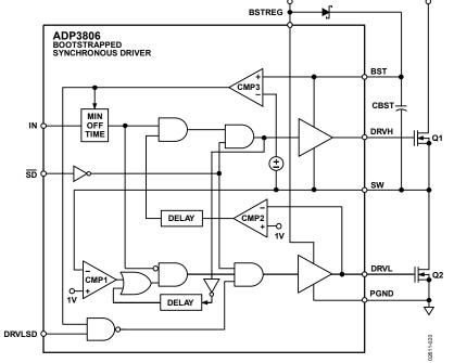
Figure 20. Bootstrapped Synchronous Driver Rev. C | Page 11 of 16
