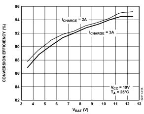
Figure 16. Conversion Efficiency vs. Battery Voltage
