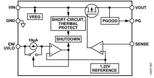
Figure 3. ADP7102 Functional Diagram
