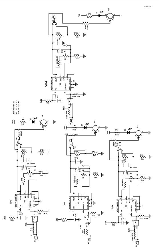
Figure 16. ADM1260 Evaluation Board Schematic, Page 4
