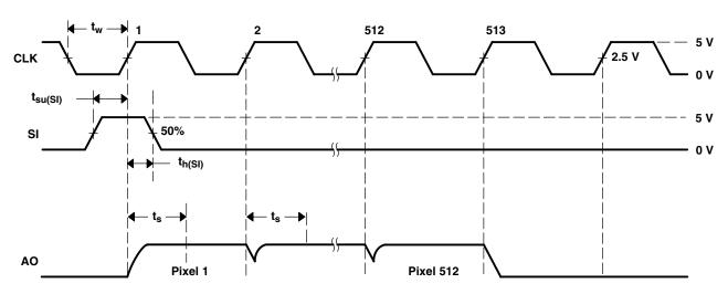
Figure 2. Operational Waveforms (each section)
