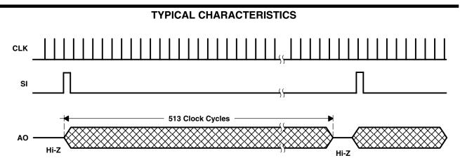
Figure 1. Timing Waveforms (each section)
