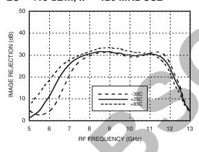
Image Rejection vs. LO Drive, IF = 120 MHz USB
